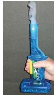
FIGURE 16: “WIZARD STICK” SMOKE GENERATOR IN USE
