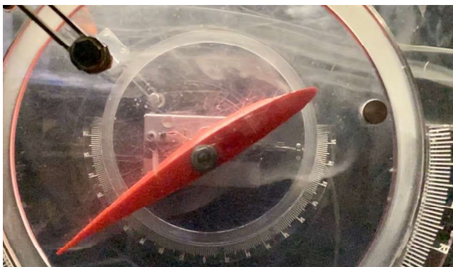
FIGURE 35: NACA 63-210 TESTING AT AOA 30 degrees.
