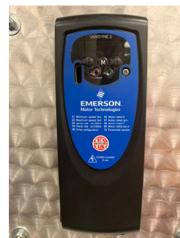
FIGURE 3: CLOSE-UP OF EMERSON MOTOR RPM CONTROLLER OF WIND TUNNEL
