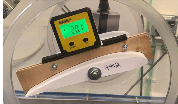
FIGURE 15: NACA 4412 IN TESTING WITH ITS CUT-OUT PLATFORM AND JOHNSON DIGITAL ANGLE GAUGE
