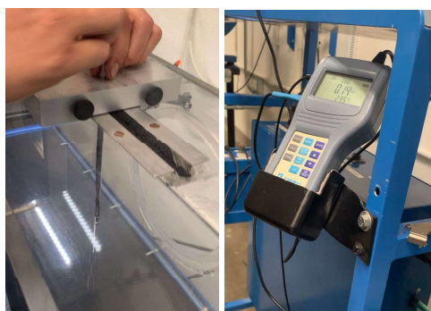
FIGURE 6: HOT-WIRE, SPECIAL HOLDER, TEST SECTION SLIDERS, AND ANEMOMETER
