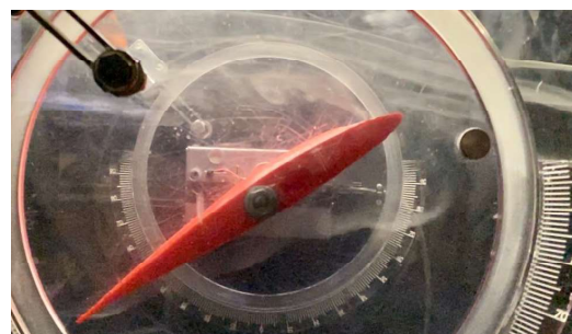
FIGURE 17: VORTICES REPRESENTED VISUALLY BY GENERATED SMOKE ABOVE NACA 63-210 AIRFOIL TILTED 30 DEGREES
