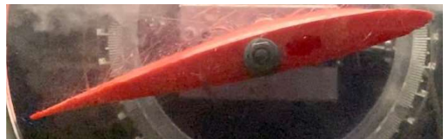
FIGURE 13: NACA 63-210 3D PRINTED AIRFOIL BEING TESTED
