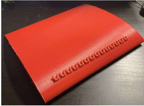
FIGURE 14: NACA 63-210 3D PRINTED AIRFOIL WITH VORTEX GENERATORS
