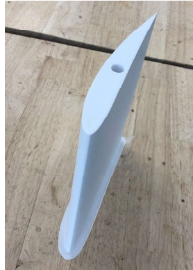
FIGURE 11: NACA 4412 3D PRINTED AIRFOIL BEFORE POLISH
